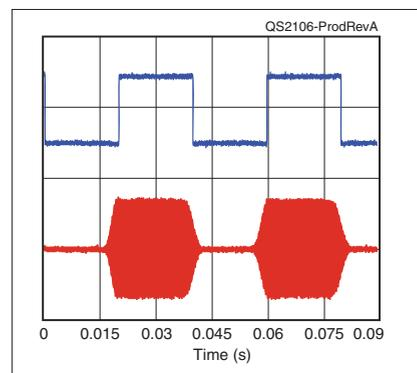
**Figure A** — The CW keying waveform for the Yaesu FTDX10, showing the first two dits in full-break-in (QSK) mode, using external keying and the default 6-millisecond rise time setting. Equivalent keying speed is 60 WPM. The upper trace is the actual key closure; the lower trace is the RF envelope. (Note that the first key closure starts at the left edge of the figure.) Horizontal divisions are 10 ms. The transceiver was being operated at 100 W output on the 14 MHz band.
