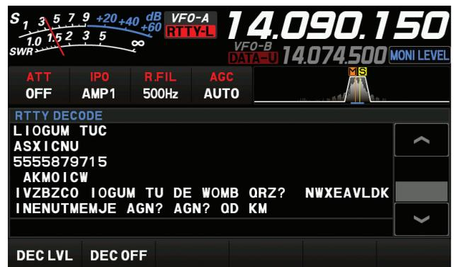
**Figure 4** — During the BARTG RTTY Contest, the FTDX10's RTTY decoder tries to render readable text, but with mixed results. The passband display to the right of the AGC indicator shows mark and space frequencies to aid in tuning.
